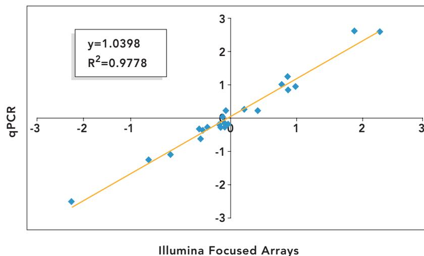
Log-log plot showing comparison of Illumina Focused Arrays expression ratios to qPCR.
