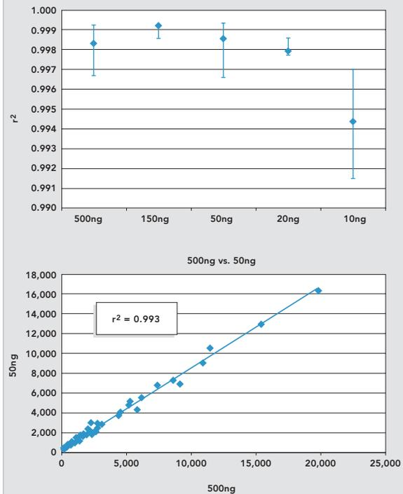
Top: Mean (diamond) and range (error bars) values are plotted for each correlation. Bottom: Correlation between sample preparations from different starting amounts of total RNA. The linear correlations for the hybridization signals of expressed RNA represented on the array were calculated for all pairwise comparisons at each starting material point.
