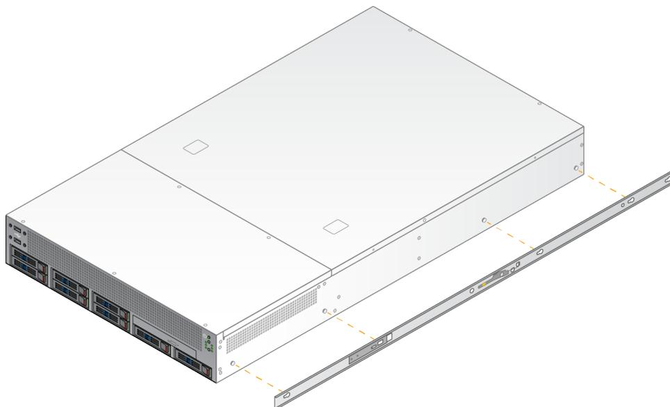
4. Repeat to attach the mounting bracket on the other side.
