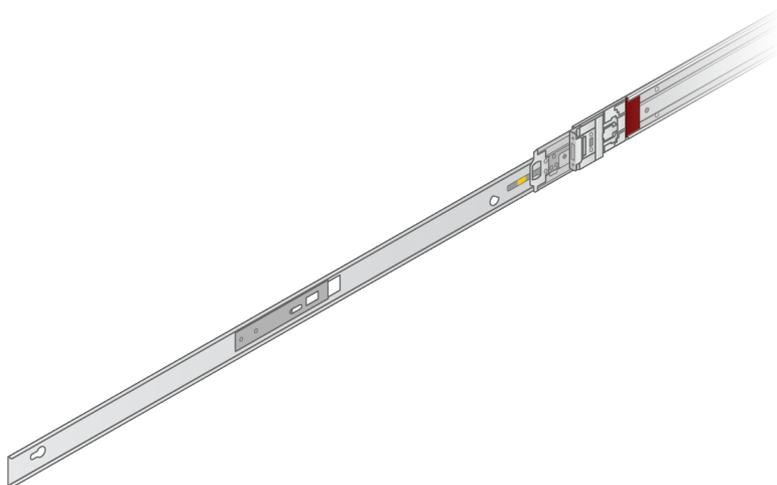
3. Align the key slots to the T studs on the sides of the server and slide the mounting bracket back to lock into place.
