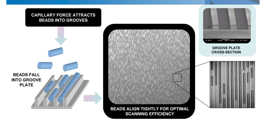
Each bead is read three times: one pass reads the barcode, two others read the green channel and red channel intensities
